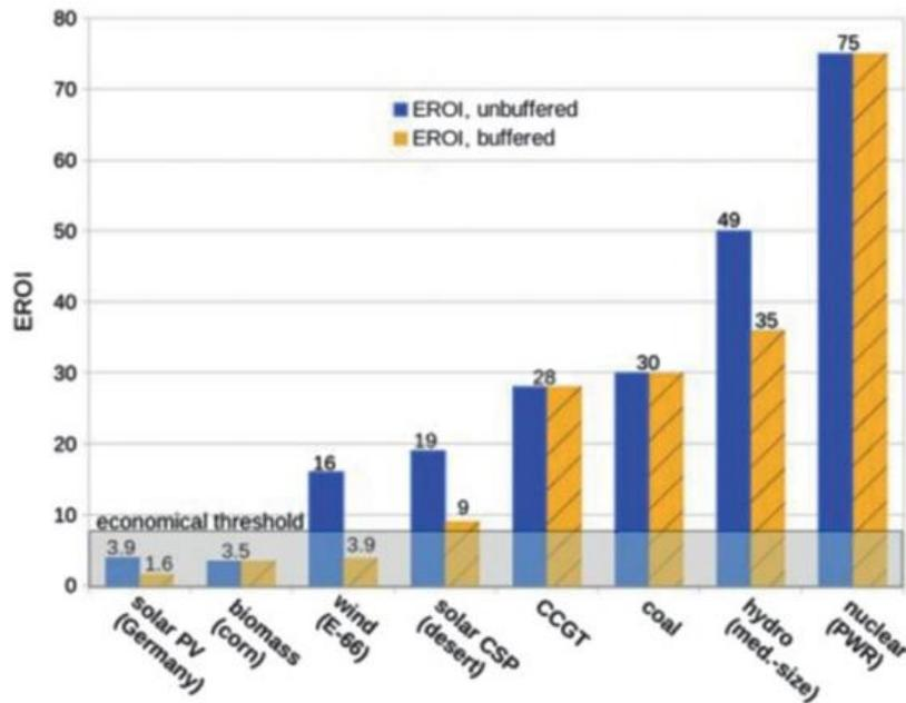
**Figure 2.** The energy return on energy invested for various forms of energy generation with the threshold for supporting a modern economy indicated across the bottom.<sup>23</sup> The advantages of fossil fuels and nuclear energy are very clear. Reprinted from Ref. 23, with permission from Elsevier.
